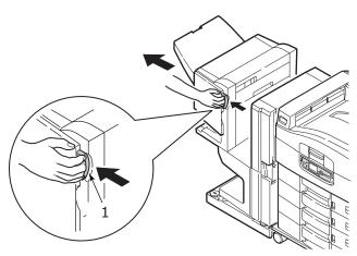
**2.** Squeeze the recessed handle (2) and open the left side cover of the Inverter.
